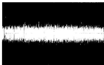
Tracking signal P108 pin 4 V: 20mV/div H: 0.5mS/div
