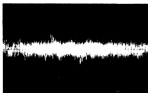
Focusing signal P108 Pin2 V:10mV/div. H:0.5ms/div.
