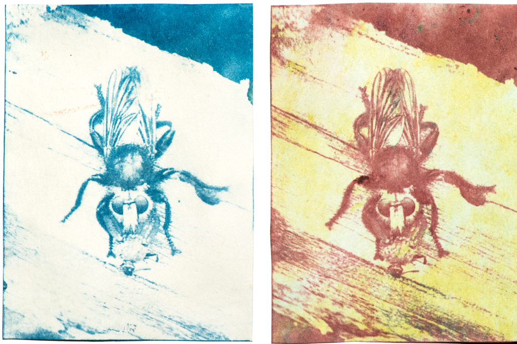
Figure 2. Cyanotype print with dimensions 8 \times 11 \text{ cm}^2 ( 3.15 \times 4.33 \text{ in}^2 ) (light source, 20 W blacklight CFL; exposure time, approximately 1.5 h) compared to a svinotype print (light source, 75 W incandescent light bulb; exposure time, 5 min) from the same negative image.
