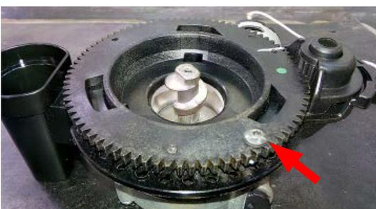
The new machines have a coffee grinder with the screw to prevent the disassembly of the upper coffee grinder support (see photo).
