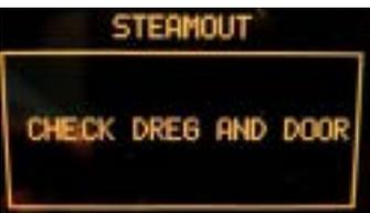
**IMPORTANT NOTE:** to execute the Steam-Out procedure the DREGDRAWER must be in place and the DOOR must be closed. If these 2 conditions are not respected a warning message is shown on the display and the Steam-Out is interrupted
