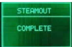
When the Steam Out is complete the message "COMPLETE" is shown on the Display. The Electro valves automatically closes and the machine can be switched off.
