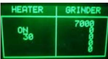
**Press the Z1 button to switch on the Heater**
