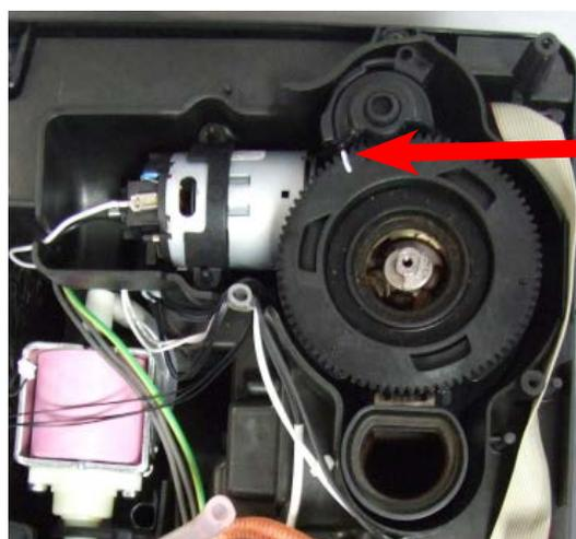
For a standard adjustment, both markings must be aligned.
