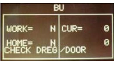
**Press the Z1 button to move the BU to Work**
