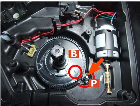
Replace the gear (B), making sure that the imprint of the arrow is aligned with the opening containing the pin (P).
