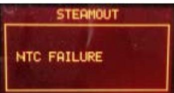
**IMPORTANT NOTE:** to execute the Steam-out procedure the Ntc sensor must work correctly; if some errors occurs on Ntc during the steam-out, the procedure can't continue and an error message is shown on the display.
