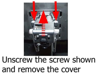
Unscrew the screw shown and remove the cover
