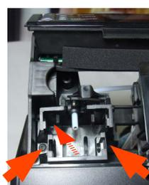
Loosen the screws holding the carafe connection
