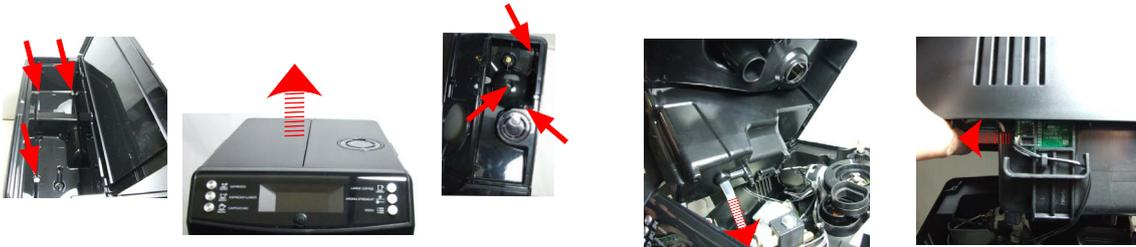
Unscrew the screws shown, raise the top cover and remove the electrical and water circuit connections.
