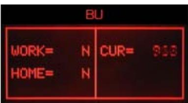
**ERROR: (With BU)** The absorbed current is higher than 300mA, the display backlight changes from green to red; check the BU and the motor
