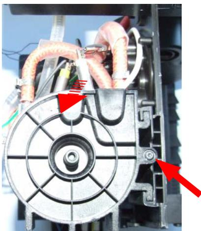
Unscrew the screw shown at unthread the support boiler
