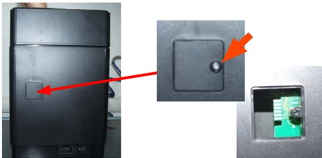
Loosen the screw for remove the cover.
