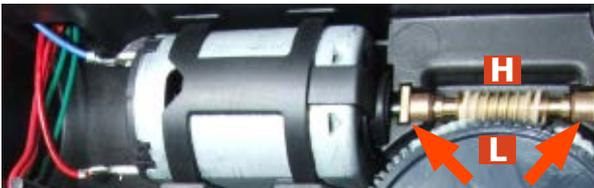
When replacing the motor and the transmission shaft, make sure the guide runners (L) are in the right position.
