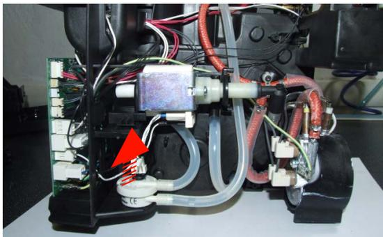
Lift the flow meter out of the casing assembly and remove the electrical and water circuit connections.
