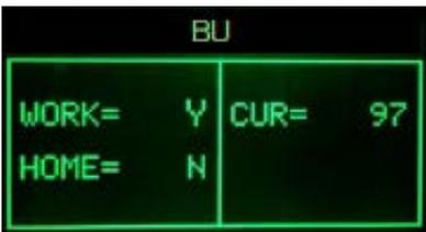
When the BU reaches the work position the indication **WORK** changes from "N" to "Y", the number of the current is less than 200mA (without BU) or 300mA (with BU).
