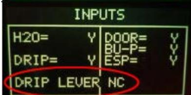
**Warning:** if the Lever sensor is not connected to interface will appear a warning message.
