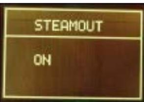
The machine starts the Steam Out and the display change the backlight (yellow) and appears the indication "ON". While the Steam Out runs the Electro valve is opened and water comes out the Water/Steam pipe.
