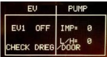
**Press the Z1 button to open the Electro Valve**
