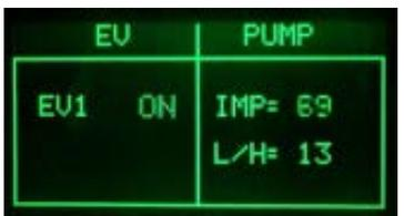
**Press and Release the Z4 button to switch on the pump (100 impulses)**
