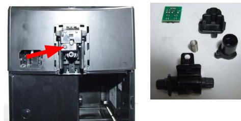
Unscrew the screw shown and remove the cover
