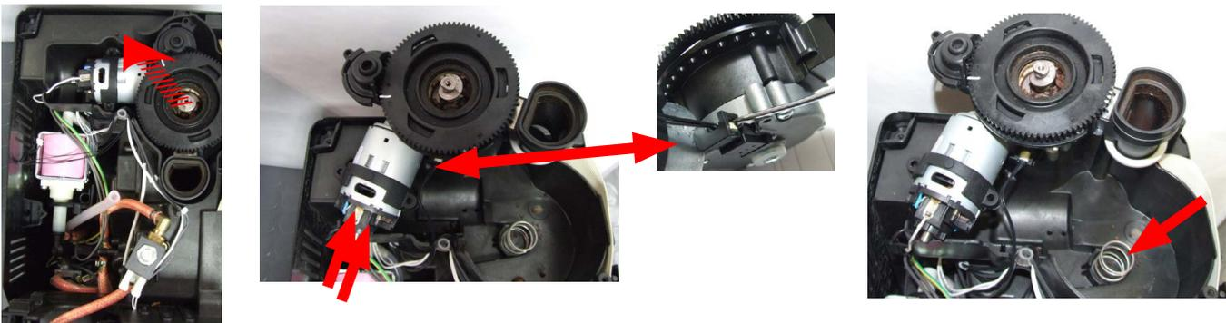
Raise the coffee grinder and remove the connections.
