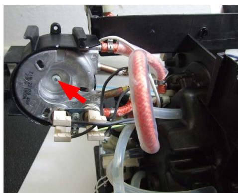
Unscrew the screw shown and remove the electrical and water circuit connections.
