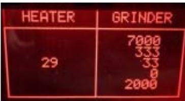
**ERROR:** The number remains 0 or the grinder does not run, or the display backlight changes from white to red; check the Grinder and the wiring from the Grinder to the CPU/POWER board (JP8)
