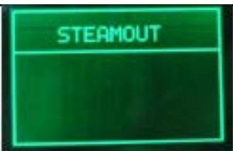
Once entered the Steam Out mode the display shows the "STEAM OUT" indication. Buttons can be released
