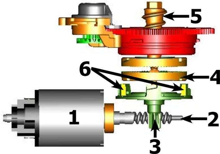
The coffee grinder is driven by a direct current motor (1) using a worm screw helicoidal wheel transmission (2).
